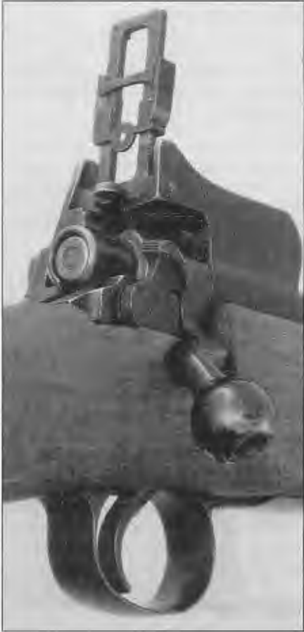
Rear sight assembly, adjustable for elevation but not windage.
