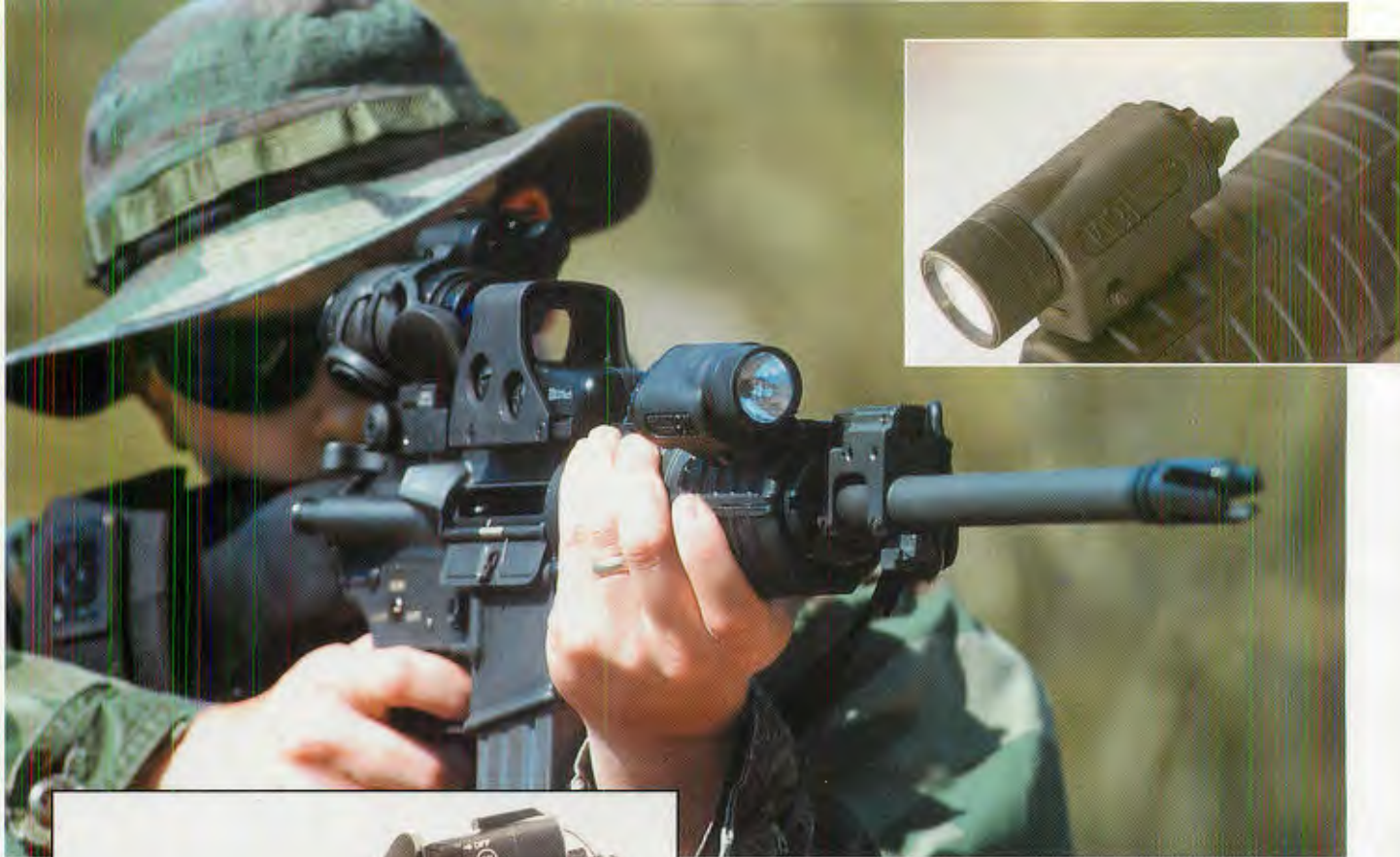
(top, inset) The M3 Tactical Illuminator weighs only 3.3 ounces with batteries. Yet, using a tungsten halogen, xenon-filled bulb and two standard DL 123A 3-volt lithium batteries, the unit delivers an amazing 80-90 lumens of white light. Shown here attached to an M16A2 by means of a GG&G mount. (left) Right now, the hottest optical sight combination available for the tactical M16/AR-15 series may very well be the new EOTech Model 500 Holographic Diffraction Sight with a Litton M983 night vision scope mounted to the rear.
